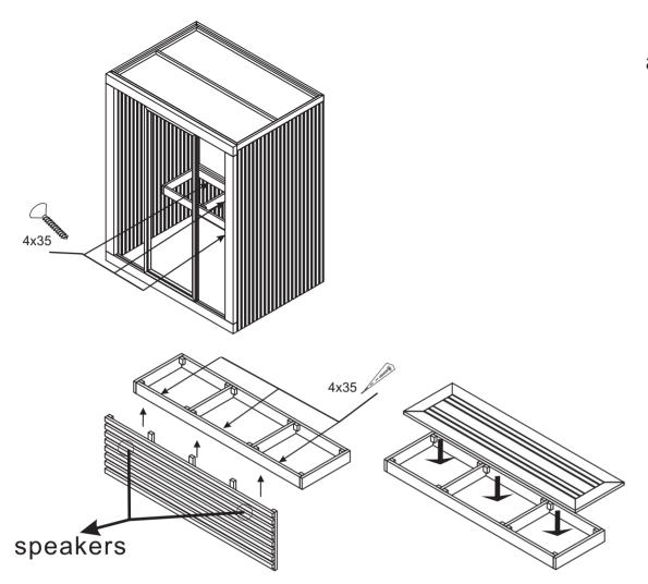
6.Seat installation. Lock the seat frame & seat back fence by screws. Put it in the seat place. The whole seat frame should be on the same horizontal line. Install 2 speakers at the back side of seat back fence (as drawing). After that, lock the whole part on the back board. (in package top board & seat board & its support)
